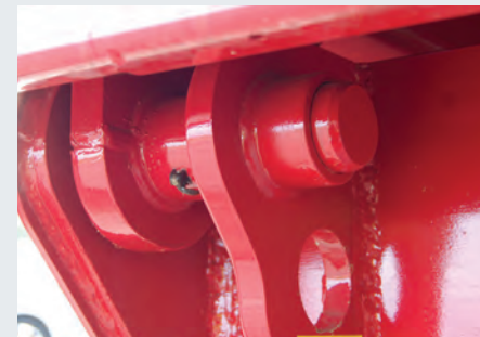
(50mm fully-bushed tip point and rear tow point)
