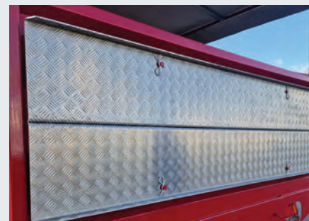
(Disabled access ramp in storage location)
