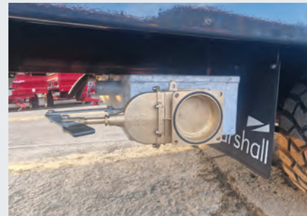
(Slurry tank valve)
