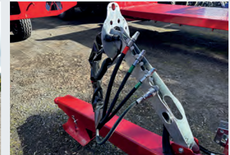
(Hydraulic hose identifiers, hose protector and detachable electrical suzi)
