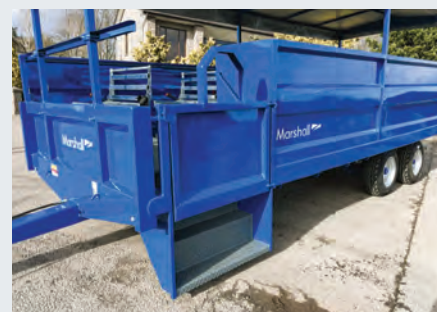
(Low level access step and safety gate)
